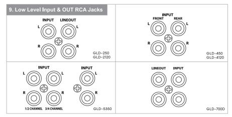
These inputs are for signal cables from the source. Always use high quality shielded RCA cables. The LINE OUT allows you to build multiple amplifier systems without having to use splitter cords to distribute the signal. Now it is simply a matter of bringing one set of RCAS into the first amplifier, then using the line out RCA jacks as the feed to the next amplifier.
