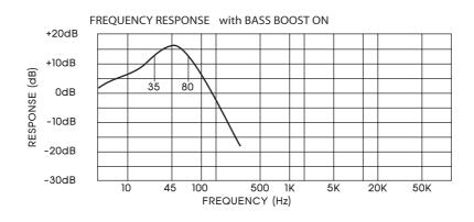
NOTE: Raising the Bass Frequency allows higher frequencies to reach the bass speakers centered around 45Hz. This "BUMP" can have a dramatic effect on the bass system's apparent volume. Use caution! When adjusting this control as serious subwoofer damage may result from overpowering or overexcursion.
